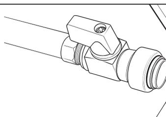
mark pipe exterior at 1" depth required for proper fit
